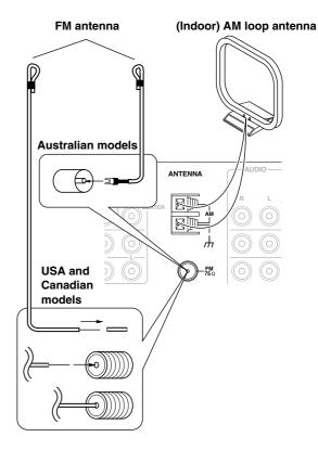
Strip away the insulation from the end of the cable, and fully insert the stripped end of the cable.
